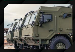
The armoured cabins of the TDV company have the same interior design as the standard nonarmoured cabins of Tatra vehicles, including the instrument panel and control elements, so the transition between the two types of cabins does not pose any problem for the crews. In addition, armoured cabins have special seats that protect the crew from the effects of mine explosions and explosive devices under the vehicle.
